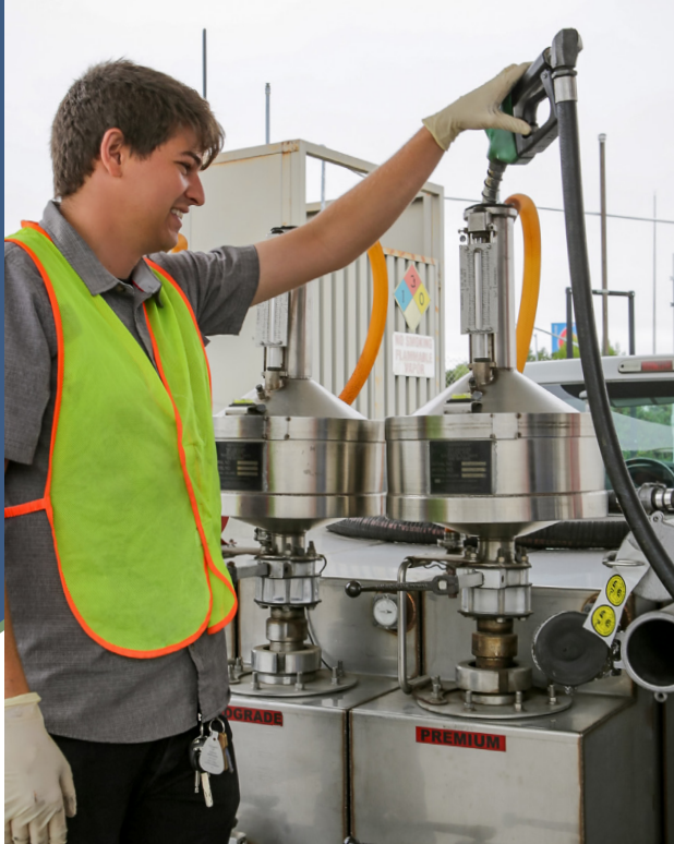
Above: An inspector verifying retail fuel meter (gas pumps) accuracy.
