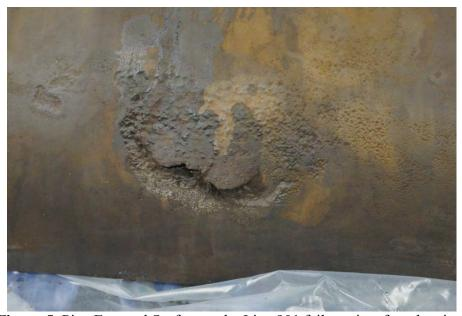
Figure 5. Pipe External Surface at the Line 901 failure site after cleaning.
