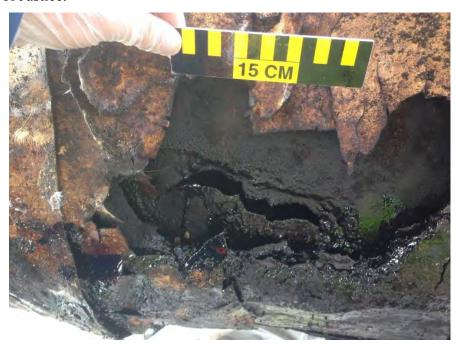
Figure 4. The failed pipe and surrounding insulation and coating.
