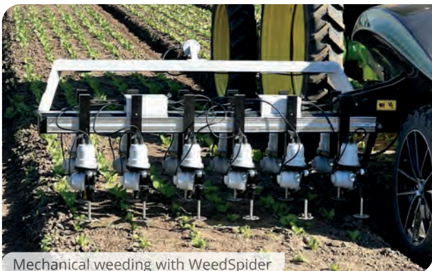
Mechanical weeding with WeedSpider
